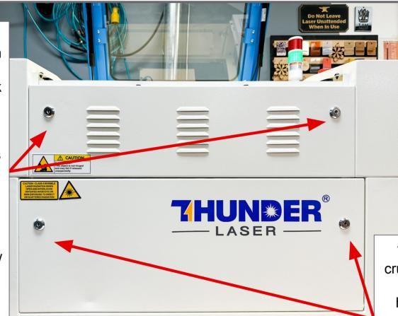
This is the door for the crumb tray, and where you would remove the honeycomb. Unlike the passthrough door, it's held on with a spring hinge. Please still be careful and don't let it drop against the machine
