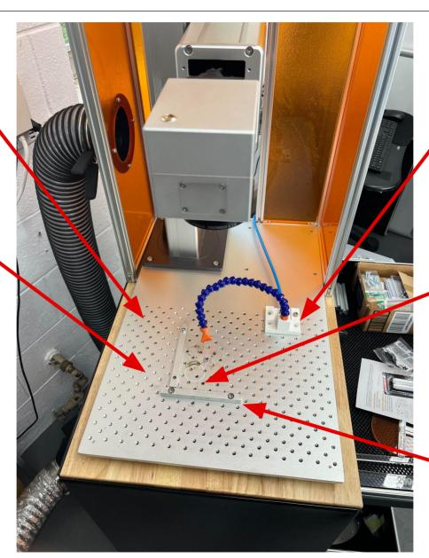
The air assist base can be moved around the bed and kept in place with one or more M6 screws.
