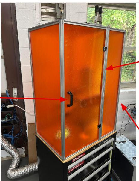
The case is in two parts so that the front half can be taken off to accommodate large parts. There are latches on the front and back to hold both parts of the enclosure tightly together.
