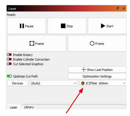
Each lens is set up as a different device. You must change the Device to match the lens focal length you are using. There are only two choices and they are labeled with the focal length.
