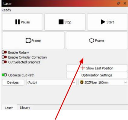
There is no option to change the origin point. The origin point is always the middle focus point of the laser.
