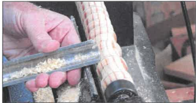
14. Presented on its side, the SRG quickly flattens beads in preparation for cutting coves.
