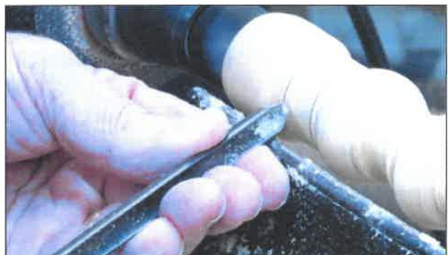
16. The cove cut starts with the gouge on its side, flute pointed towards the cove interior.
