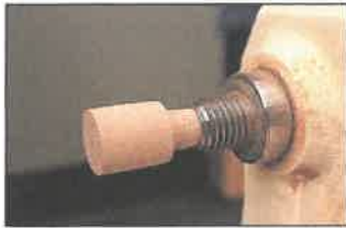
Spinning top blank with turned Morse taper secured in headstock
