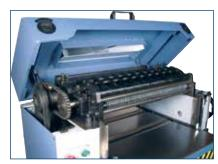
EASY ACCESS TO CUTTERHEAD keeps maintenance time to a minimum.
