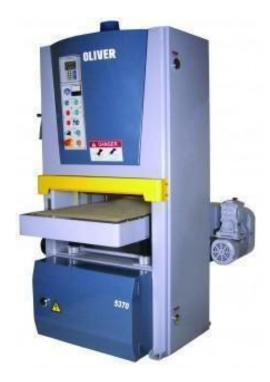
**What is it used for?** The wide belt sander is used for finish sanding wide panels such as cabinet doors, cabinet face frames, panels that are glued up of several pieces of wood and other wide flat panels.
