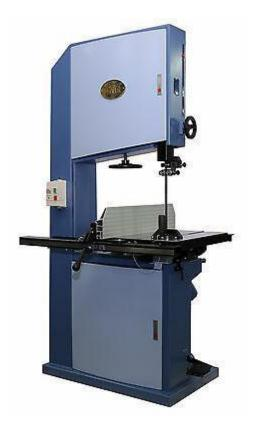
What is it used for? Band Saws come in a variety of sizes from small handheld machines to very large machines used for cutting up logs. Our machine falls in the middle and is intended to be used in a woodworking shop on lumber that has already been dried and cut into rough dimensional sizes. It is set up to cut wood, plywood, manufactured wood products like MDF or Masonite and some soft materials like plastic.
