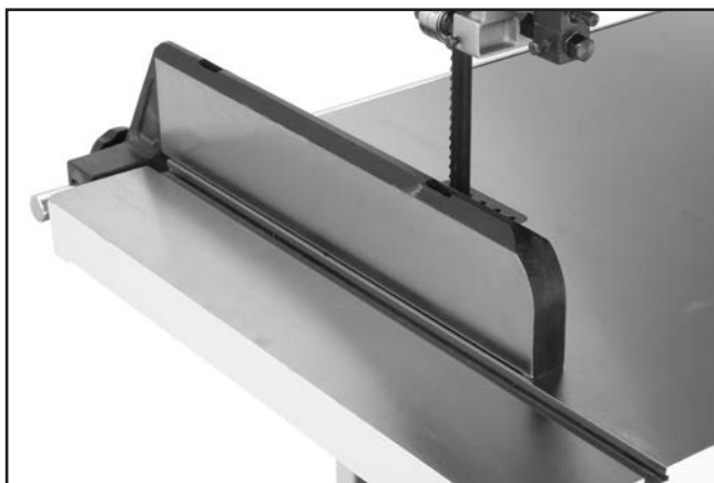
Figure 61. Example of fence parallel with miter slot.
