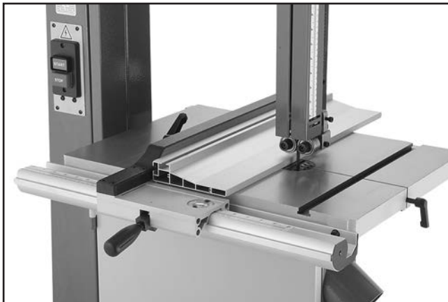
Figure 80. Resaw fence installed in the alternate position.
