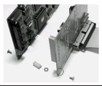
Insert the Daughter Board on to the 40-pin connector of the PCI-7200 card. Attach the two cards with the included spacer, washer, and screws. This will insure constant connection between the two boards.
