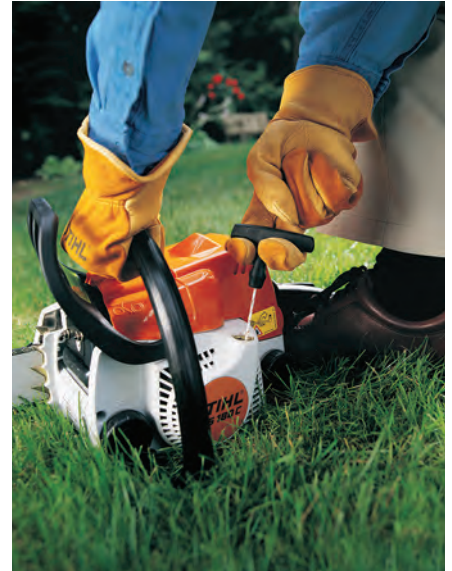
Hold your chainsaw firmly on the ground when starting. Handheld starts are dangerous because you risk losing control.
