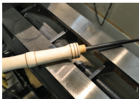
This tool handle is not safe. Include a ferrule when you make your own tool handles so that the wood will be supported near the shank of the tool. For this tool handle, which was turned too small for the available ferrule, I will attach a small hose clamp.
