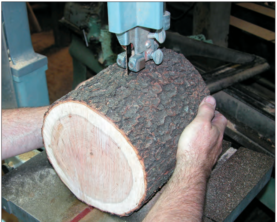
A recommended ripping procedure: The downward pressure of the bandsaw blade reduces the tendency of the log to roll side to side.
