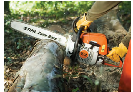
A chainsaw is safest when used near ground level. Never use a chainsaw above shoulder height.
