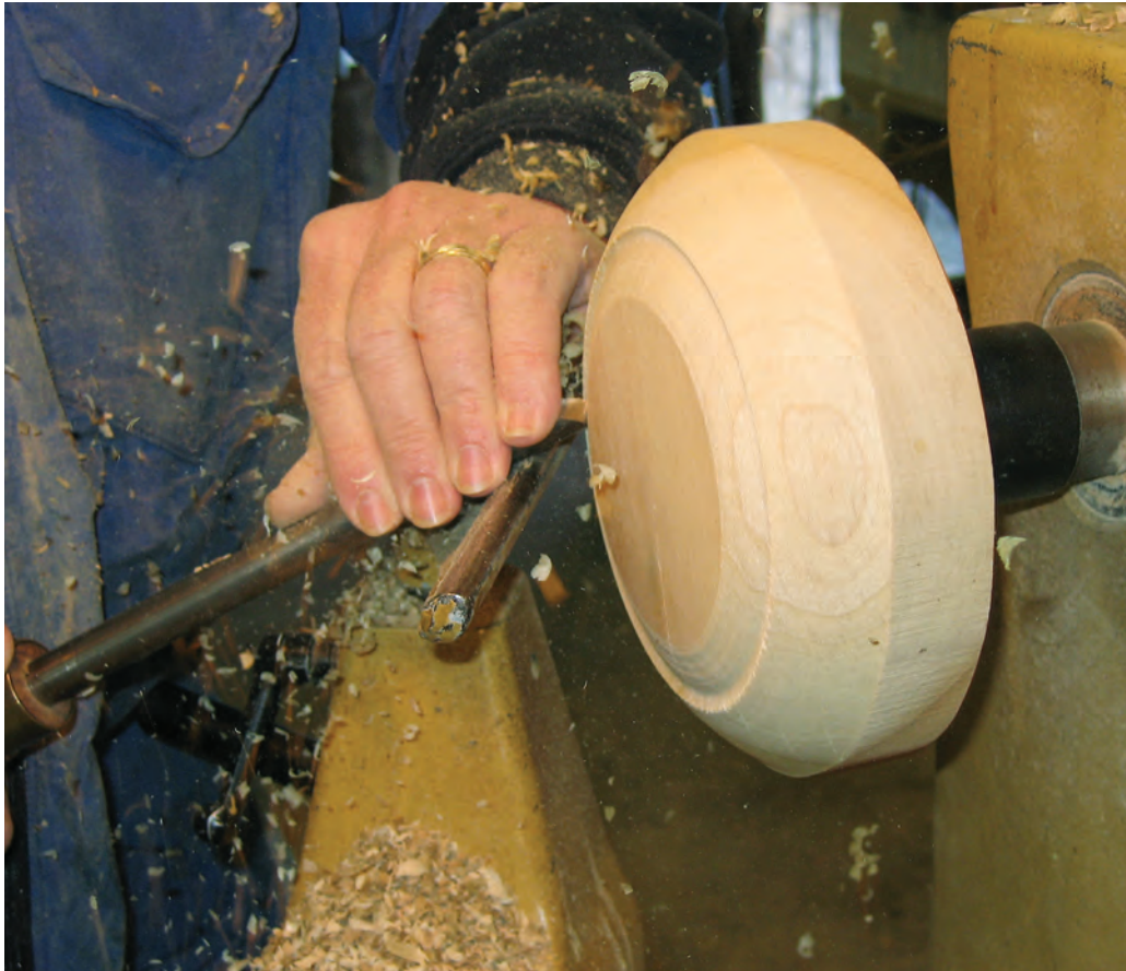
When turning the outside of a face-grain bowl, turn from the bottom to the top (sometimes described as uphill).
