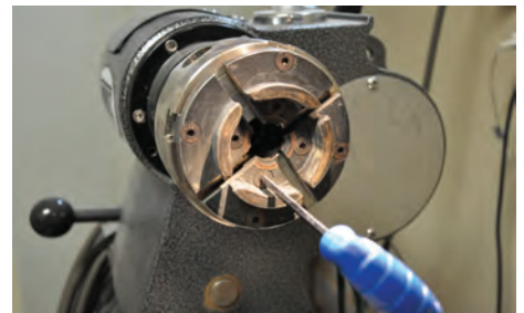
Tighten the hex screws that attach the jaws to the body of the chuck.
