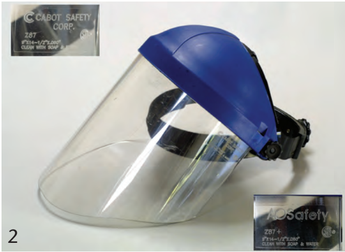
2 This faceshield has a thick polycarbonate shield. Note the impact rating in the inset images, basic impact, Z87 (upper left) and high impact, Z87+ (lower right).
