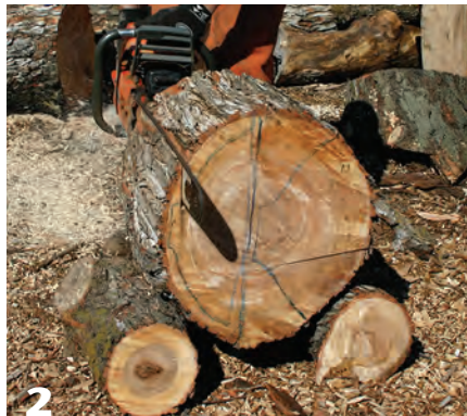
2 After marking both ends of the log, make the first cut through the 18"-long log.
