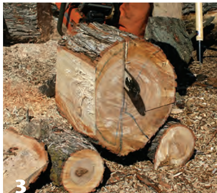
3 Separate the two blanks. Note how the log is elevated to keep the chain out of the dirt.
