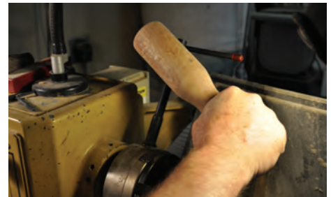
Secure your chuck (or faceplate) onto the lathe’s spindle either by hand or use a mallet if you are not strong enough to push it tight. I use the mallet method, which I learned from one of the older turners.
