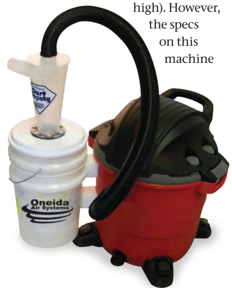
The Dust Deputy from Oneida turns an ordinary shop vacuum into a two-stage unit, where the larger particles are sent to the bucket and the fines are trapped and collected in the unit's standard bin.
