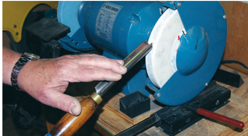
Potential danger: Using a long fixture arm and a blunt sharpening angle brings the tip of the tool too close to the wheel's equator. If the arm of the jig slips or too much pressure is exerted, it could cause the tool to jam against the wheel.
