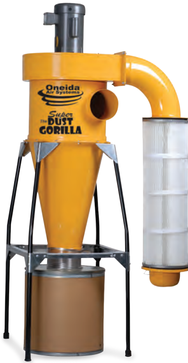
Combining the benefits of cyclone separation with an exterior two-stage filter and a large debris bucket, the 2 HP Super Gorilla from Oneida is a unit well suited to turners who take on larger bowl projects, and therefore need more than one dust port.
