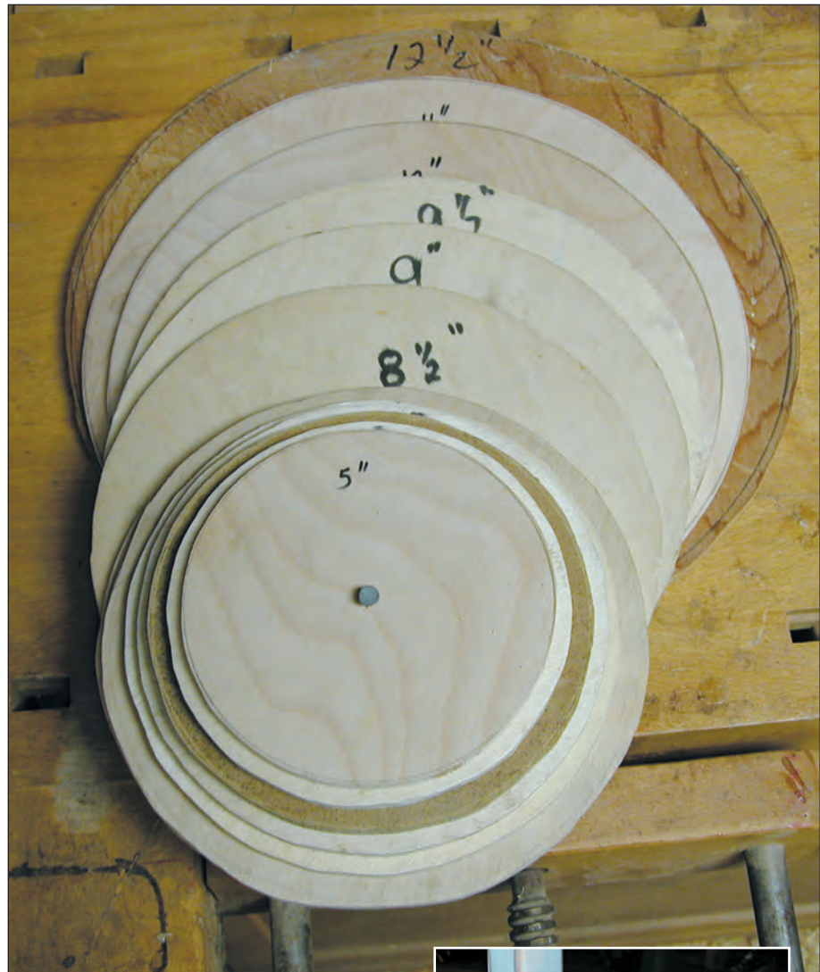
Spend a few minutes to make a set of cutting patterns, shown above, for your lathe's swing capacity. The 8" pattern is shown at right on a birch log.
