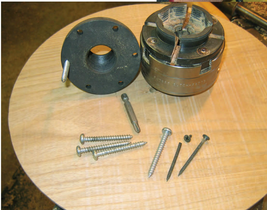
Sheet-metal screws should be your only choice for mounting turning stock to faceplates. At right , you can see how a drywall screw can break off, which leads to huge safety issues.
