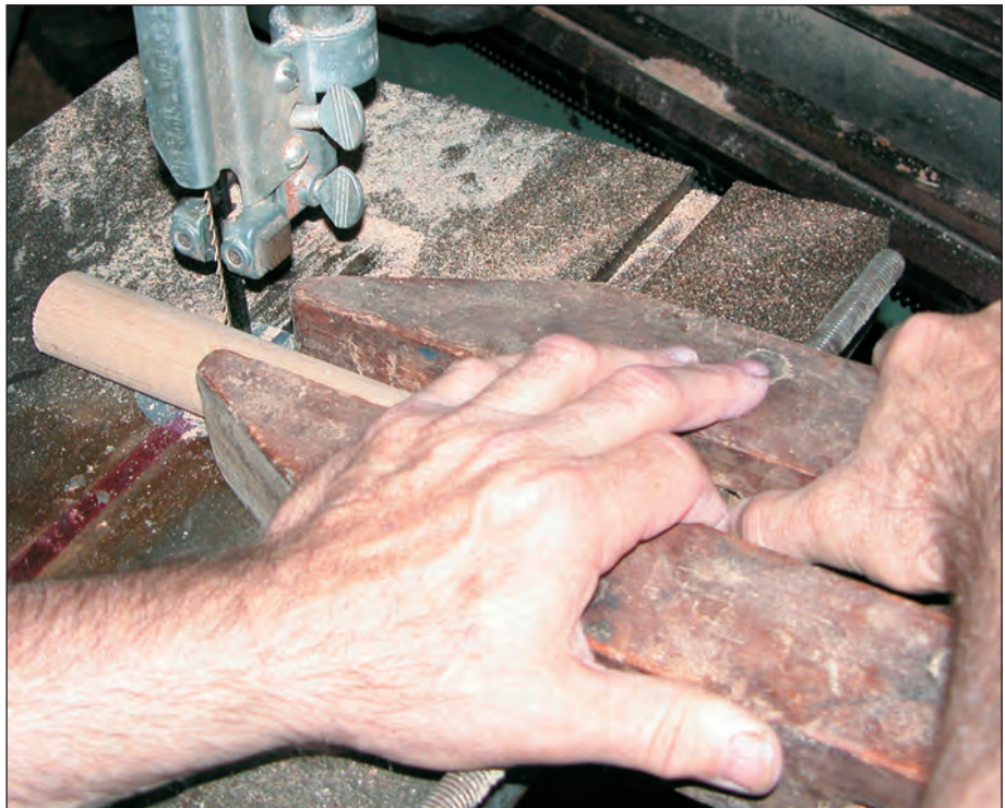
To crosscut short round stock, securing material in an adjustable parallel (handscrew) clamp is a solid solution.
