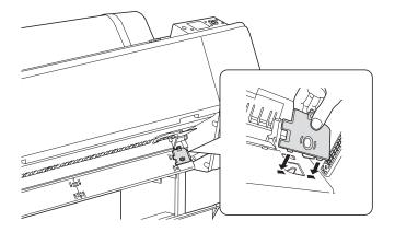
7. Install the SpectroProofer in the printer by sliding it onto the mounting rails.
