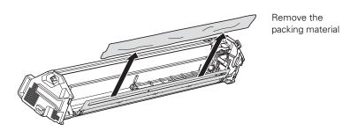
3. Remove any packing tape from the carriage.
