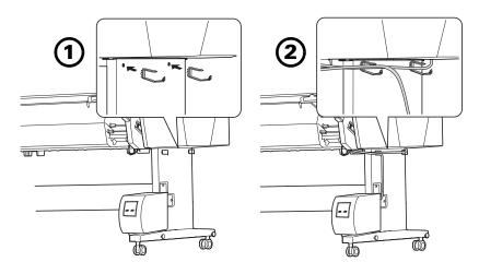
5. Plug the SpectroProofer's USB cable into the option port on the back of the printer.
