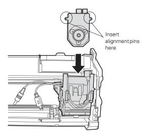
Connect the cables on the carriage to the spectrophotometer.
