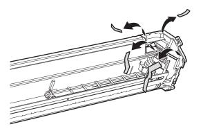
4. Remove the packing material from the cables on the carriage.
