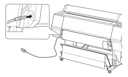
7. Attach the remaining cable hook to the inside left leg of the printer stand. Place the power cord in the hook, and snap the hook closed.
