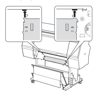
For the 44" model, attach the first backing plate on the right side of the printer, then attach the second backing plate to its left. Make sure the plates hook together as shown. Ensure that both plates rest flush against the printer and don't move when you try to slide them.
