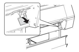
3. Using the included bolts and Allen wrench, install the mounting rails in the two locations shown below.
