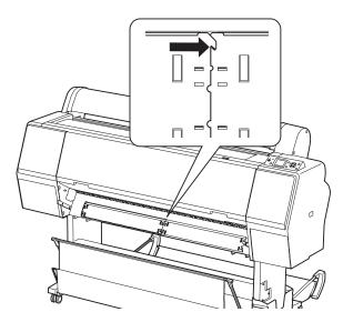
5. Insert the calibration tile into the holder. Remove the cover on the back of the holder by rotating it. Drop in the tile with its white surface face-down. Replace the cover.
