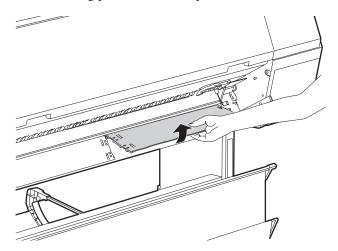
6. Use a soft, lint-free cloth to clean any dust or dirt from the surface of the calibration tile and backing plate(s).
