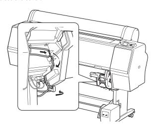
4. Attach two cable hooks to the right leg of the printer stand. Place the cable(s) in the hooks as shown, and snap the hooks closed.
