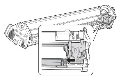
8. Insert the spectrophotometer into the carriage so it clicks into place and then insert the two alignment pins.
