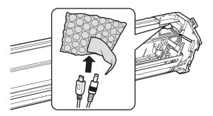
5. Slide the carriage a little to the left and then remove its plastic retainer.
