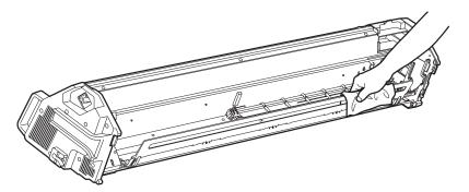
9. Lower the paper presser, then slide the carriage against it to lock it in place.
