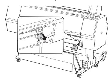
4. Remove the calibration tile from the holder.
