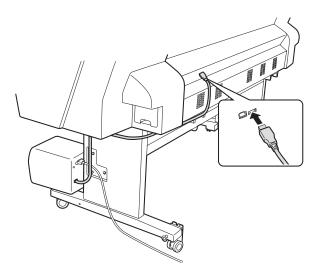
6. Plug the included power cord into the socket on the left side of the SpectroProofer.
