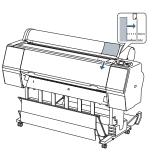
**Note:** If the sheet is more than 19 mil thick, you need to use the <sup>\*</sup>/<sub>2</sub>, Paper release (ePlaten) button.
