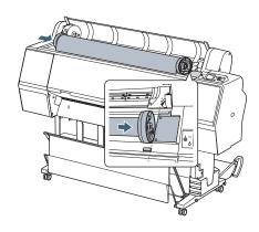
7 Slide the roll paper holder to align the left adapter with the ▲ on the holder.
