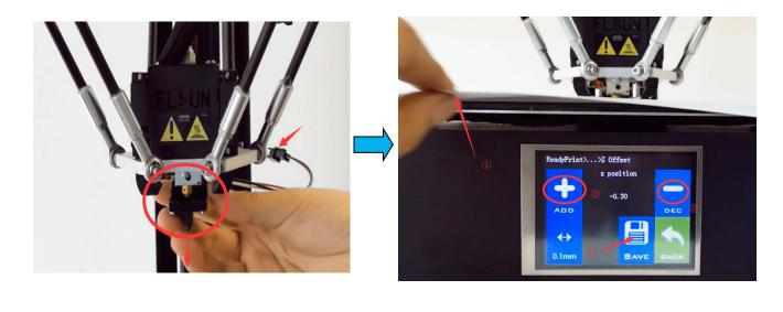
3.Remove leveling switch module before click Move\_Z0 button.
