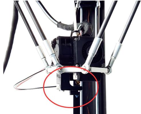
2. **Plug** in leveling switch module before auto-level, notice that the Line must be plugged
