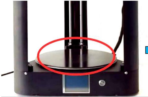
1. **Clean** the glass platform before automatically leveling.
