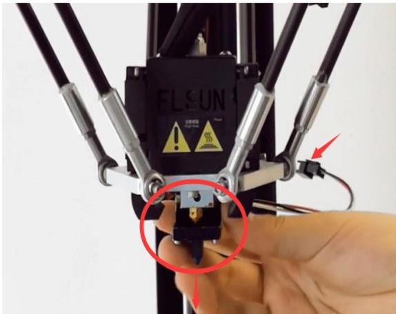
3. **Remove** leveling switch module before click **Move\_Z0** button.
