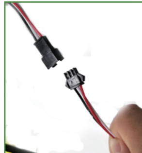
Connecting the autolevel sensor
