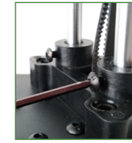
Tighten axis fixing screws of bottom shell
