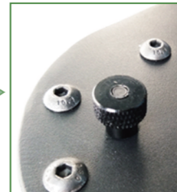
Make screw head and nut are at the same height
