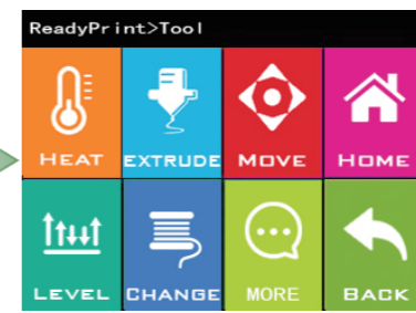
Click LEVEL → Autolevel (When autoleveling, In order to ensure the accuracy of data , the nozzle moves very slowly)
