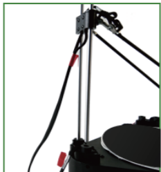
Insert optical axis through slider to shaft seat bottom
