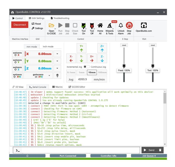
Use the Jog Buttons (X, Y, and Z arrows) to move the torch to a reasonable starting place and raise the Z axis enough to fit your material under it. (You will likely want continuous jog. Slide the switch to the right. It will move as long as you hold the button down.)
