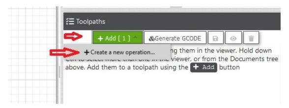
A line of icons will be added in the Toolpaths window and the Configure Toolpath window will appear.
