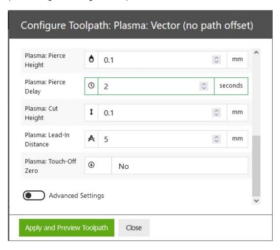
Note: Pierce Height and Cut Height must be greater than zero
