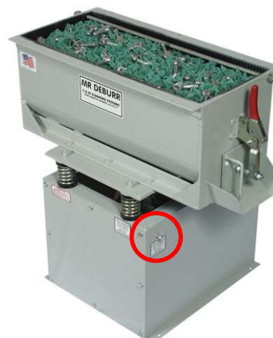
Figure 3: Bearing Grease Zerk Fitting Circled
