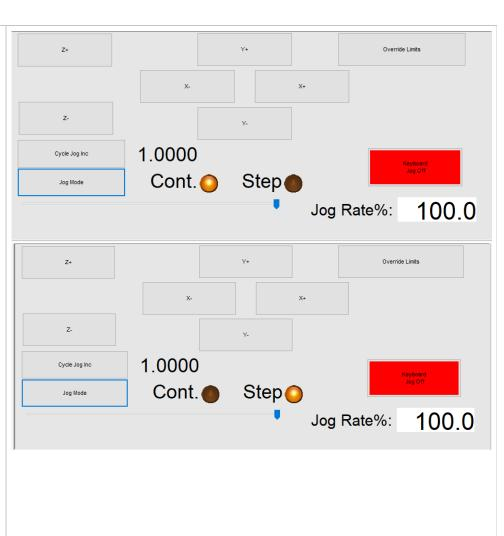
If you have Jogged the machine to far and you hit an endstop that machine will be disabled and you cannot jog that machine without overriding the machine by selecting the Override limits button.
