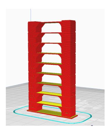
Using the slider on the right side of the screen, find the point at which the first section of the tower ends and the second section begins. Make note of the layer number
